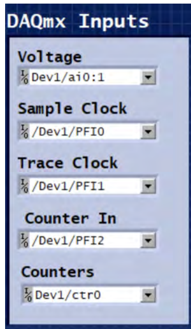
Figure B.2: The DAQmx Inputs typedef in the experiment control code allows users to designate which channels of the NI USB-6212 data acquisition device are used for different functions.
