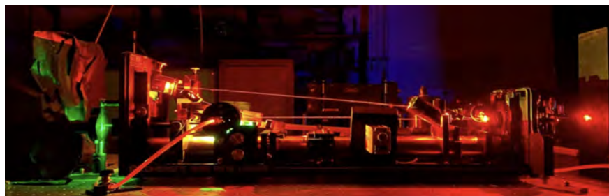
Figure 2.5: Photograph of our Coherent 899 CW Dye Ring Laser in operation. The laser’s wide tunability throughout the visible region and narrow linewidth make it advantageous for high-resolution spectroscopy.
