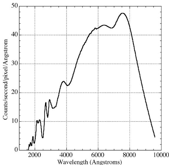
Fig. 4. TRACE “White Light” instrumental response to an un-limb darkened solar spectrum.
