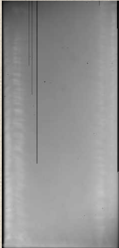
Flat field exposure of an EEV42-80 CCD
