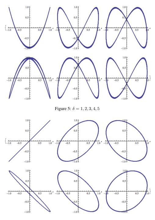
Figure 6:  $\frac{\omega_x}{\omega_y}=1.0$  with  $\delta=0,1,2,3,4,5$
