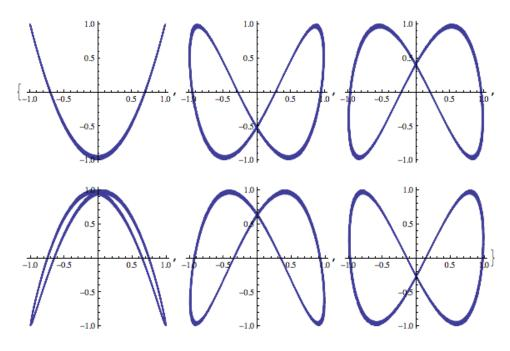
Figure 8:  $\frac{\omega_x}{\omega_y} = 2.0$  with  $\delta = 0, 1, 2, 3, 4, 5$
