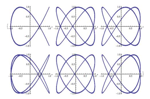
Figure 7:  $\frac{\omega_x}{\omega_y} = 1.5$  with  $\delta = 0, 1, 2, 3, 4, 5$
